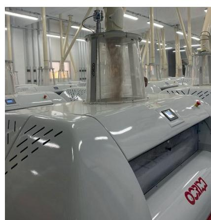
The plant - tested in March 2021 - for processing common wheat has a capacity of 600 T/24h and produces two types of flour: boulangerie, for baking, and patisserie or beignet, with a low ash content, for pastry or special applications. Important flours - especially boulangerie - for the agro-food industry and the needs of the African continent.
